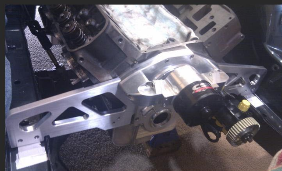
CUSTOM ENGINE PLATE FOR HOLDEN V8 WITH BILLET COVER. PLATE MOUNTS MECHANICAL FUEL PUMP, DRY SUMP PUMP & VAC PUMP.
